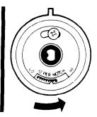
4. To raise the temperature, move a notch closer to HI. Each notch equals about 10°F (5°C).
